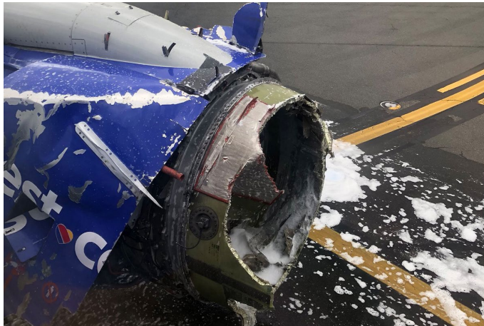
Fatigue failure of turbine blade 1 person killed
