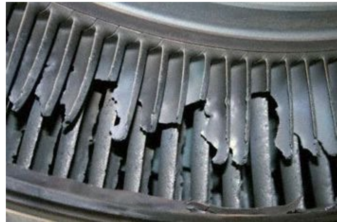
Excessive creep extension of blade, tip shroud/seal interference and blade rupture
